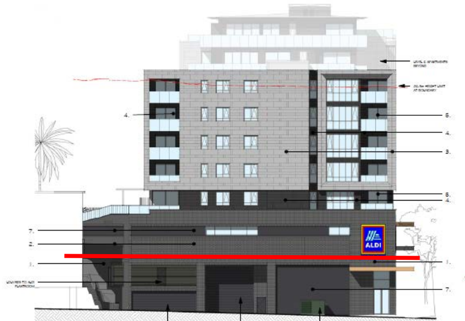
Figure 7: Rear elevation of proposal – red line denotes ceiling level of loading area, most of which is excluded from definition of GFA but adds to the height and bulk of the building
